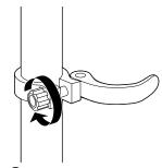
**3** The tension of the quickrelease clamping mechanism can be adjusted by tightening or loosening the bolt with your fingers.
